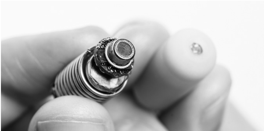
Figure 16.2 Photograph of the open capsule, showing the electronic circuit, sensors, packaged batteries and coil antennae (left) and the packaged capsule (right)
